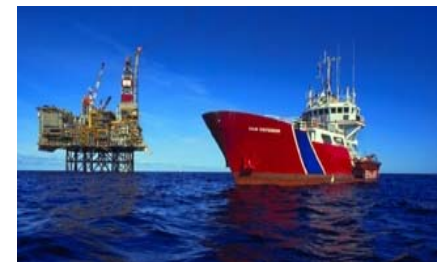
Laser controls boat position to oil rig
