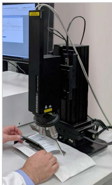
Figure 1 - A Virsa fibre-probe on its motorised stage, being used to analyse a turbine blade from an aircraft engine. The blade measured approximately 200 mm × 100 mm × 80 mm.
